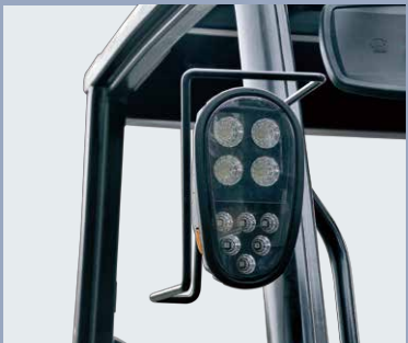
The new efficiency lighting system employs LED illuminant and new type reflector to reduce energy consumption, improve significantly illumination performance and prolong work time
